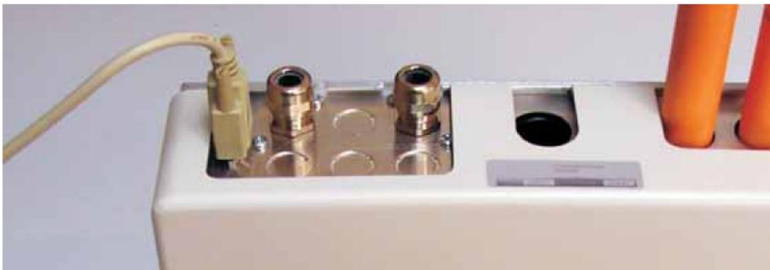
Figure 26: Connecting a PC to the command module RS-232 port
