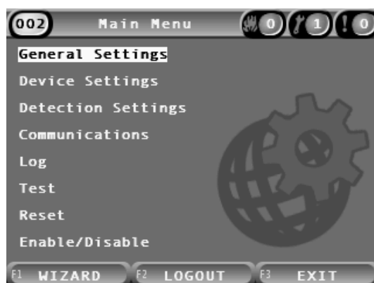
Figure 23: Access level 2 Main menu
